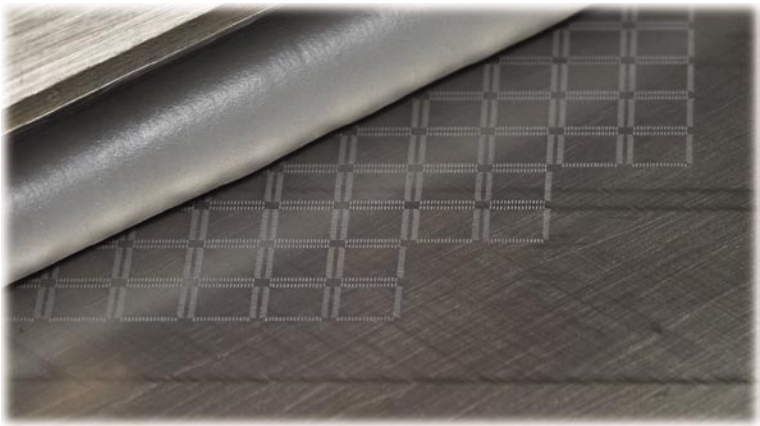
Magnified view of SE-CURE® 7101 printing on a metal foil water bumping stencil.
